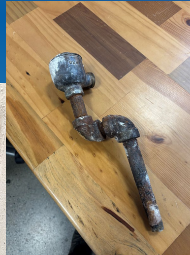
Failed condensate return pipe in library
